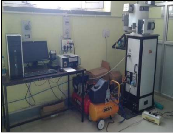
High Temperature Reciprocating Tribometer
