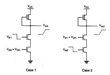
NAND2 circuit delay analysis m1 3 1 0 0 mn w=5u 1=1u m2 4 2 3 0 mn w=5u 1=1u m3 5 4 4 0 mnd w=1u 1=3u c1 4 0 0.1p cp 3 0 0.05p vdd 5 0 dc 5.0
