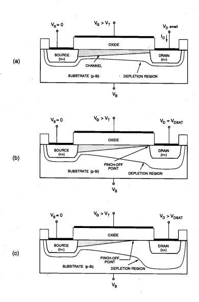
Figure 3.14. Cross-sectional view of an n-channel (nMOS) transistor, (a) operating in the linear region, (b) operating at the edge of saturation, and (c) operating beyond saturation.
