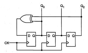
Figure 16.12. A pseudo-random sequence generator using LFSR.
