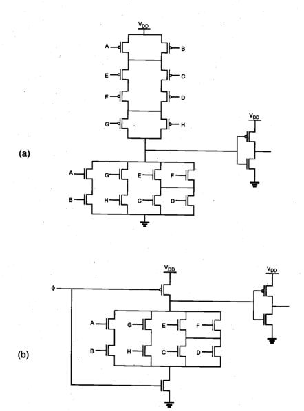
Figure 9.30. (a) An 8-input complex logic gate, realized using conventional CMOS logic and (b) domino CMOS logic.
