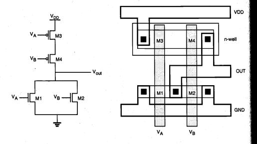
Figure 7.14. Sample layout of the CMOS NOR2 gate.
