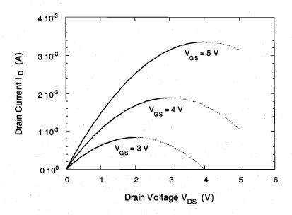
The drain current-drain voltage curves shown above reach their peak value for  $V_{DS} = V_{GS} - V_{T0}$ . Beyond this maximum, each curve exhibits a negative differential conductance, which is not observed in actual MOSFET current-voltage measurements (section shown by the dashed lines). We must remember now that the drain current equation (3.32) has been derived under the following voltage assumptions,
