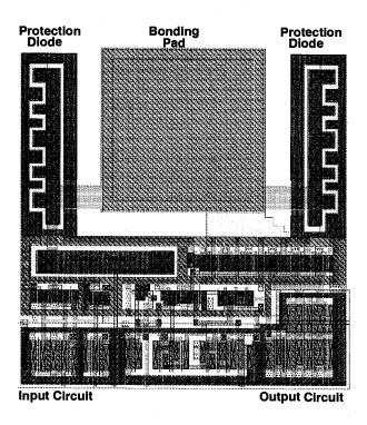
Figure 13.18. Layout of a bidirectional I/O pad circuit (courtesy of MOSIS).
