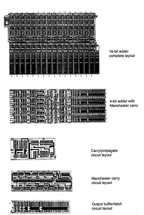
Figure 14.7. Layout of a 16-bit adder, and the components of its physical hierarchy.
