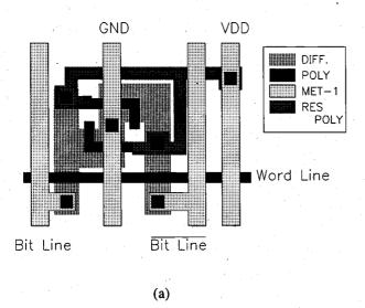
Figure 10.25. (a) Layout of the resistive-load SRAM cell.
