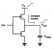
Figure 11.30. A CMOS inverter circuit with a stepwise-increasing supply voltage.
