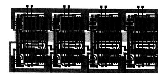
PLATE 10: (Top) Layout of a CMOS full adder (FA) circuit.
