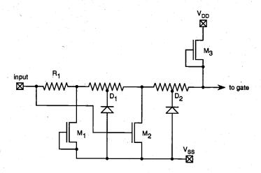
Figure 13.4. Protection network with thick-oxide transistor.
