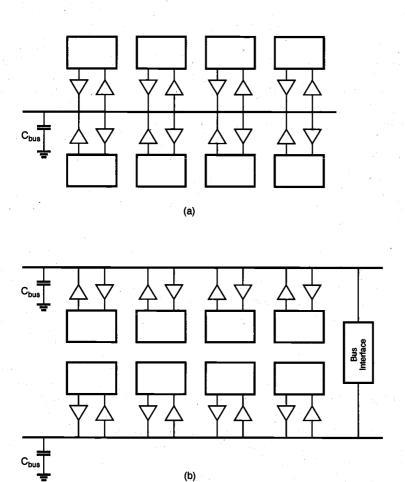
Figure 11.25. (a) Using a single global bus structure for connecting a large number of modules on chip results in large bus capacitance and large dynamic power dissipation. (b) Using smaller local buses reduces the amount of switched capacitance, at the expense of additional chip area.
