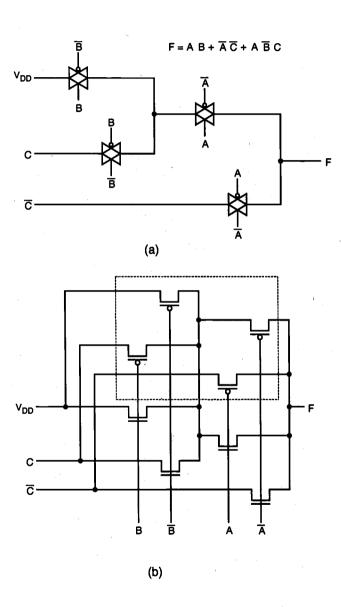
Figure 7.40. (a) CMOS TG realization of a three-variable Boolean function. (b) All pMOS transistors can be placed into one n-well to save area.
