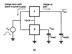
*Figure 11.28.* (a) The general circuit topology of a conventional CMOS logic gate. (b) The topology of an adiabatic logic gate implementing the same function. Note the difference in charge-up and chargedown paths for the output capacitance.
