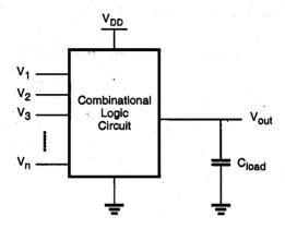
Figure 7.1. Generic combinational logic circuit (gate).
