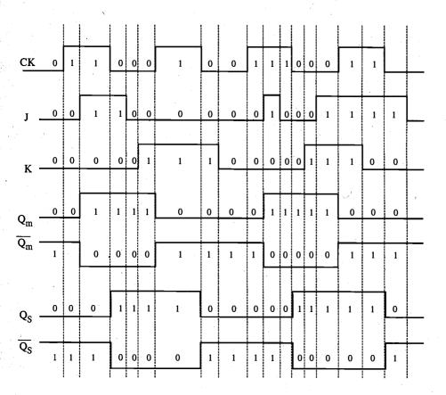
Figure 8.24. Sample input and output waveforms of the master-slave flip-flop circuit.
