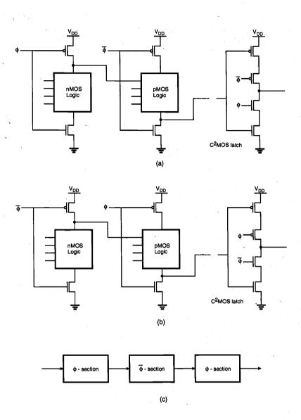
Figure 9.39. (a) NORA CMOS  $\phi$ -section; evaluation occurs during  $\phi = 1$ . (b) NORA CMOS  $\phi$ -section; evaluation occurs during  $\phi = 0$ . (c) A pipelined NORA CMOS system.
