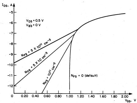
**Figure 4.7.** Variation of the drain current in the weak inversion region, as a function of the gate voltage and for different values of the parameter  $N_{FS}$ , in the LEVEL 2 model (Copyright © 1988 by McGraw-Hill, Inc.).
