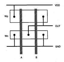
Figure 7.16. Stick-diagram layout of the CMOS NOR2 gate.
