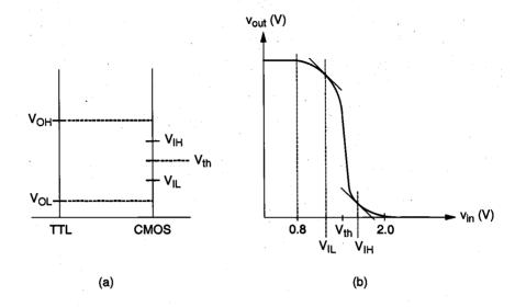
Figure 13.8. (a) TTL to CMOS level shifting and (b) the corresponding voltage transfer characteristic curve.
