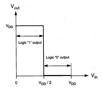
Figure 5.2. Voltage transfer characteristic (VTC) of the ideal inverter.
