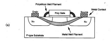
Figure 13.5. (a) Typical ESD failure modes.
