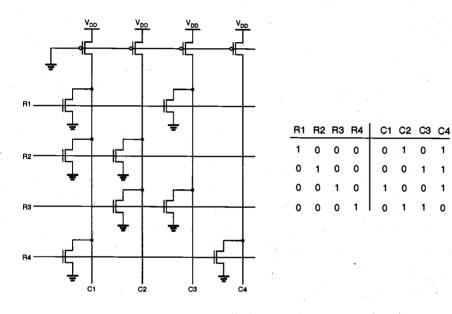
Figure 10.3. Example of a 4-bit x 4-bit NOR-based ROM array.
