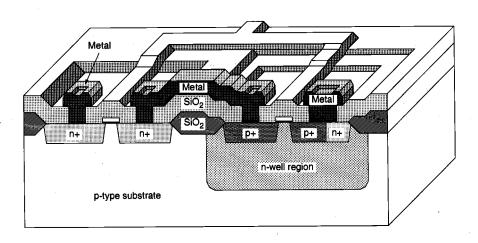
Figure 2.10. Metal (aluminum) is deposited over the entire chip surface using metal evaporation, and the metal lines are patterned through etching. Since the wafer surface is non-planar, the quality and the integrity of the metal lines created in this step are very critical and are ultimately essential for circuit reliability. After Atlas of IC Technologies, by W. Maly [1].
