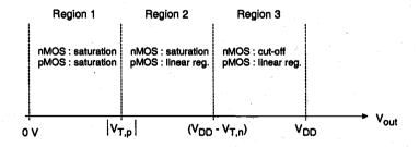
Figure 7.34. Bias conditions and operating regions of the CMOS transmission gate, shown as functions of the output voltage.
