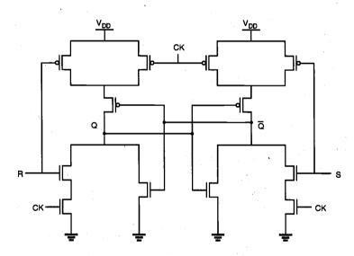
Figure 8.16. AOI-based implementation of the clocked NOR-based SR latch circuit.
