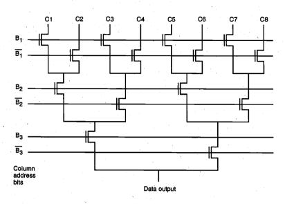
Figure 10.15. Column decoder circuit for eight bit lines, implemented as a binary tree decoder which is driven directly by the three column address bits.
