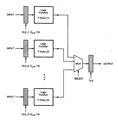
**Figure 11.17.** N-block parallel structure realizing the same logic function as in Fig. 11.15. Notice that the input registers are clocked at a lower frequency of  $(f_{CLK}/N)$ .
