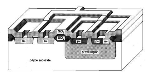
Figure 2.9. An insulating silicon dioxide layer is deposited over the entire wafer using CVD. Then, the contacts are defined and etched away to expose the silicon or polysilicon contact windows. These contact windows are necessary to complete the circuit interconnections using the metal layer, which is patterned in the next step. After Atlas of IC Technologies, by W. Maly [1].
