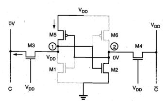
Figure 10.27. Voltage levels in the SRAM cell at the beginning of the "write" operation.
