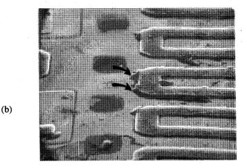
Figure 13.5. (b) SEM photograph of a failed nMOS transistor (from Reference 7).
