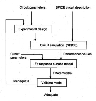
Figure 15.8. Performance modeling procedure.
