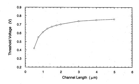
Since the conventional threshold voltage expression (3.23) is not capable of accounting for this drastic reduction of  $V_{T0}$  at smaller channel lengths, its application for short-channel MOSFETs must be carefully restricted.
