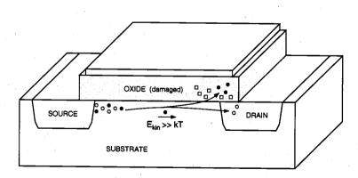
Figure 3.27. Hot-carrier injection into the gate oxide and resulting oxide damage.
