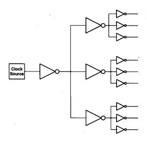
Figure 13.25. Three-level buffered clock distribution network.
