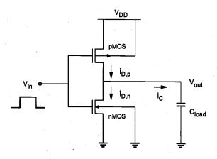
Figure 6.27. CMOS inverter used in the dynamic power-dissipation analysis.
