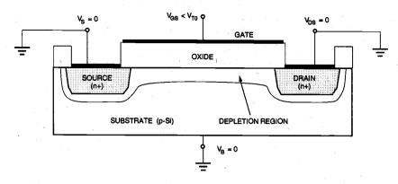
Figure 3.10. Formation of a depletion region in an n-channel enhancement-type MOSFET.
