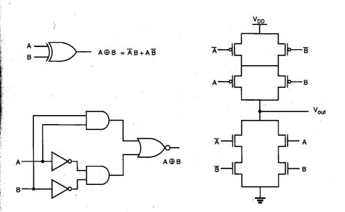
Figure 7.23. Full-CMOS implementation of the XOR function.
