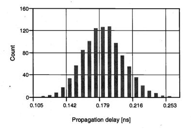
Figure 15.6. Histogram showing variation of  $\tau_P$  with  $V_{T,P}$ ,  $V_{T,P}$ , and  $t_{ox}$ .
