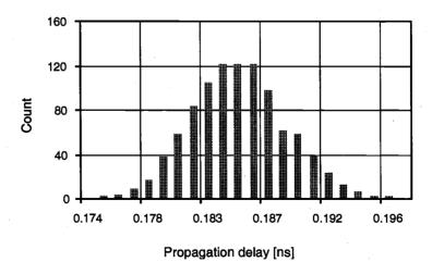
Figure 15.7. Histogram showing variation of  $\tau_P$  with  $V_{DD}$  and T. Note that the range of the distribution of delay values is much smaller than in Fig. 15.6.
