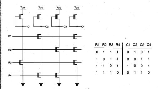
Figure 10.8. A 4-bit x 4-bit NAND-based ROM array.
