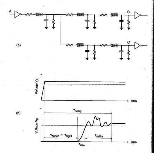
Figure 6.12. (a) An RLCG interconnection tree. (b) Typical signal waveforms at the nodes A and B, showing the signal delay and the various delay components.
