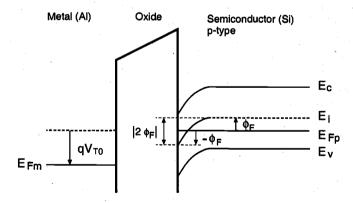
Figure 3.11. Band diagram of the MOS structure underneath the gate, at surface inversion. Notice the band bending by  $|2\phi_p|$  at the surface.
