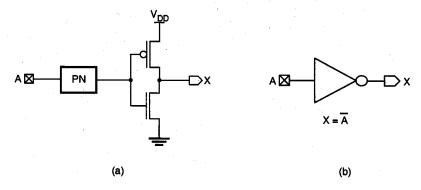
Figure 13.7. Inverting input circuit with (a) protection network, and (b) symbolic view.
