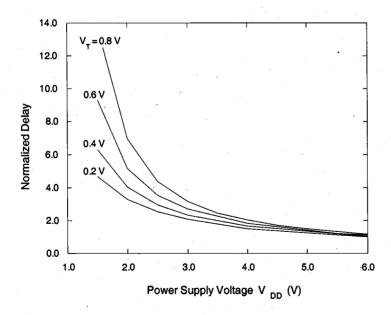
Figure 11.10. Variation of the normalized propagation delay of a CMOS inverter, as a function of the power supply voltage  $V_{DD}$  and the threshold voltage  $V_{T}$
