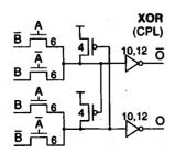
Figure 7.43. Circuit diagram of a CPL-based XOR gate.
