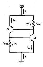
Figure 13.29. Equivalent circuit model for the SCR.
