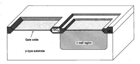
Figure 2.6. Following the creation of the n-well region, a thick field oxide is grown in the areas surrounding the transistor's active regions, and a thin gate oxide is grown on top of the active regions. The thickness and the quality of the gate oxide are two of the most critical fabrication parameters, since they strongly affect the operational characteristics of the MOS transistor, as well as its long-term reliability. After Atlas of IC Technologies, by W. Maly [1].
