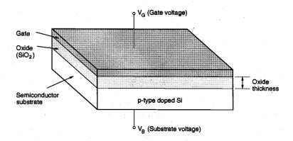
Figure 3.1. Two-terminal MOS structure.
