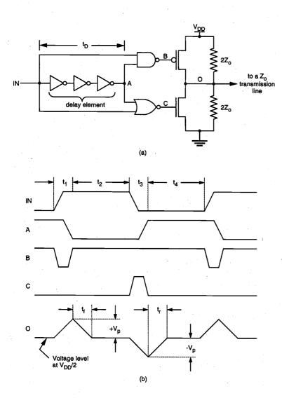
Figure 13.15. (a) Basic driver circuit that transmits only differential signals. (b) Timing diagram showing the voltage waveforms associated with the driver circuit.
