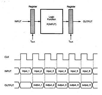
Figure 11.15. Single-stage implementation of a logic function and its simplified timing diagram.
