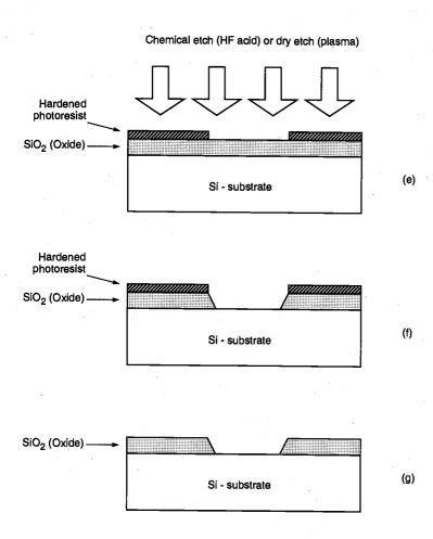
Figure 2.2. Process steps required for patterning of silicon dioxide (continued).
