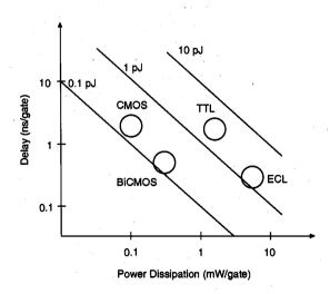
Figure 12.24. Power-delay products of BiCMOS, CMOS, and conventional bipolar logic families, using 2-µm technology.
