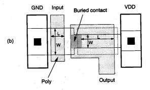
Figure 5.15. Sample layout of depletion-load inverter circuits (a) with output contact on diffusion and (b) with buried contact.
