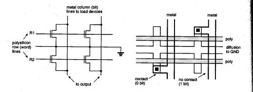
Figure 10.4. Layout example of a NOR ROM array.
