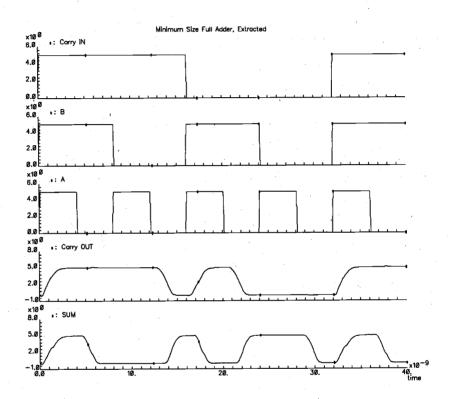
Figure 1.11. Simulated input and output waveforms of the full-adder circuit.
