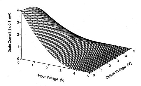
Figure 5.19. Current-voltage surface representing the pMOS transistor characteristics.
