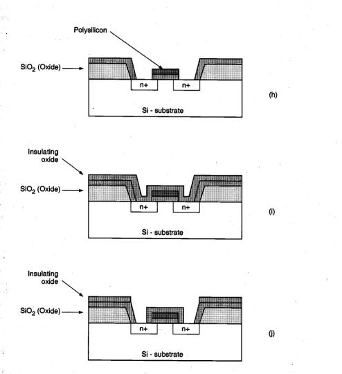
Figure 2.4. Process flow for the fabrication of an n-type MOS transistor (continued).
