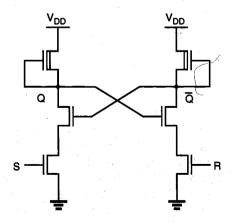
Figure 8.13. Depletion-load nMOS NAND-based SR latch circuit.
