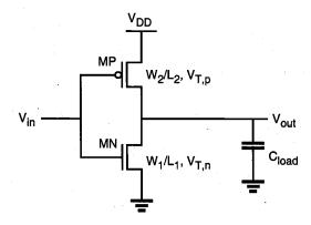
Figure 15.4. A CMOS inverter circuit.
