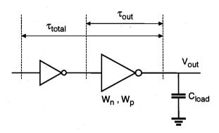
Figure 12.1. A two-stage CMOS buffer structure used for driving a large capacitive load.
