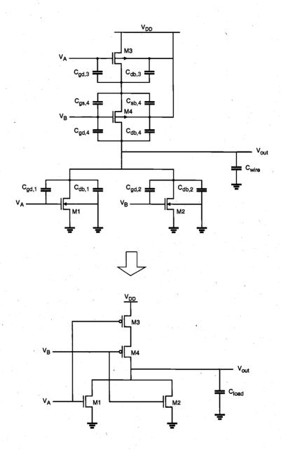
Figure 7.12. Parasitic device capacitances of the CMOS NOR2 circuit and the simplified equivalent with the lumped output load capacitance.
