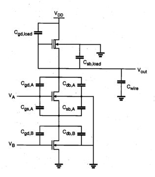
Figure 7.9. Parasitic device capacitances in the NAND2 gate.
