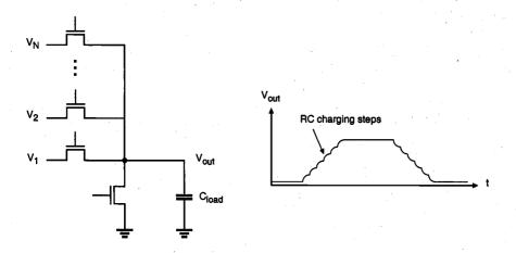
Figure 11.32. Stepwise driver circuit for capacitive loads. The load capacitance is successively connected to constant voltage sources V, through an array of switch devices.
