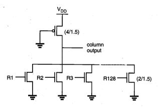
Figure 10.19. 128-input NOR gate representation of a column (bit line) in the ROM array.
