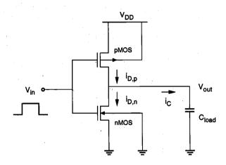
Figure 6.2. First-stage CMOS inverter with lumped output load capacitance.
