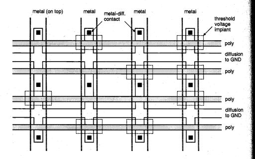
Figure 10.7. Layout of the 4-bit x 4-bit NOR ROM array example shown in Fig. 10.3. The threshold voltages of "1"-bit transistors are raised above  $V_{DD}$  through implant.
