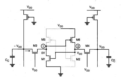
Figure 10.26. Voltage levels in the SRAM cell at the beginning of the "read" operation.
