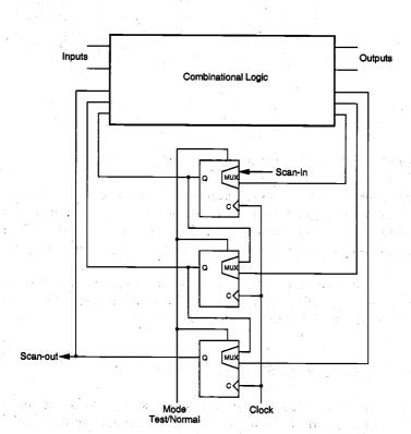
Figure 16.9. The general structure of scan-based design.
