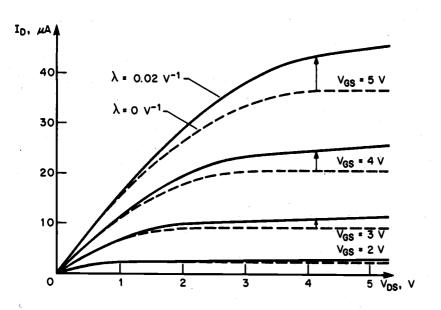
Figure 4.5. Variation of the drain current with parameter LAMBDA, for the LEVEL1 model (Copyright © 1988 by McGraw-Hill, Inc.).
