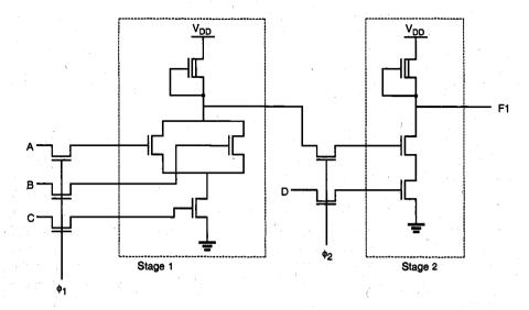
Figure 9.18. Depletion-load nMOS implementation of synchronous complex logic.
