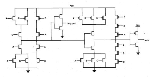
Figure 1.9. Alternate transistor-level schematic of the one-bit full-adder circuit (note that the nMOS and pMOS networks are completely symmetric).
