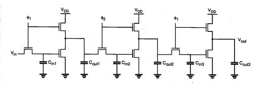
Figure 9.21. Enhancement-load dynamic shift register (ratioless logic).
