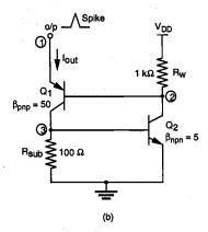
Figure 13.30. CMOS inverter circuit used in the latch-up simulation example.
