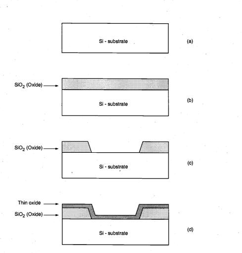
Figure 2.4. Process flow for the fabrication of an n-type MOSFET on p-type silicon.
