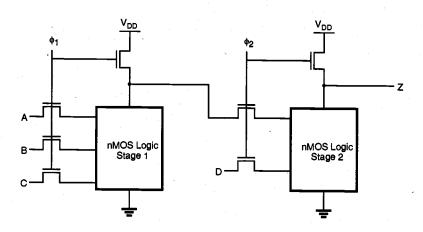
Figure 9.22. General circuit structure of ratioless synchronous dynamic logic.
