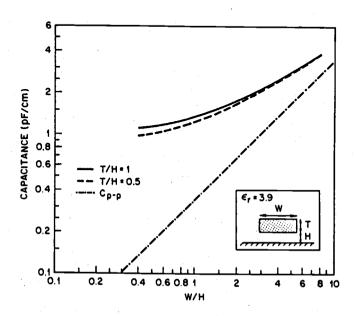
Figure 6.19. Capacitance of a single interconnect, as a function of (w/h) and (t/h).
