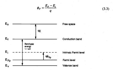
Figure 3.2. Energy band diagram of a p-type silicon substrate.
