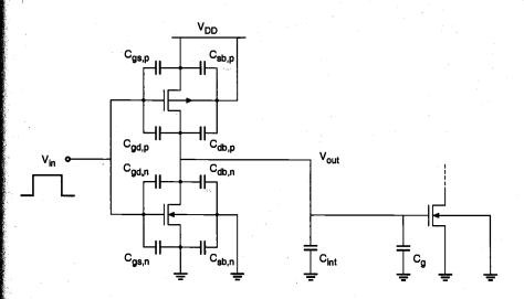
Figure 6.1. Cascaded CMOS inverter stages.
