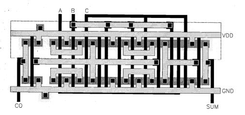
Figure 1.10. Initial layout of the full-adder circuit using minimum-size transistors.
