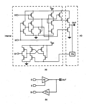
Figure 13.17. (a) Circuit diagram of a bidirectional buffer circuit with TTL input capability. (b) Block diagram of the bidirectional buffer.
