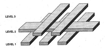
Figure 6.15. An example of six interconnect lines running on three different levels.
