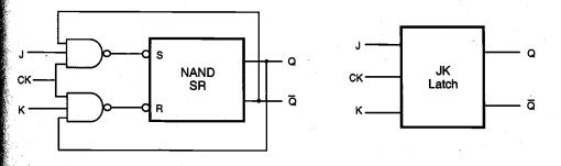
Figure 8.19. Gate-level schematic of the clocked NAND-based JK latch circuit.
