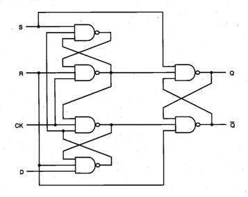
Figure 8.34. NAND3-based positive edge-triggered D flip-flop circuit.
