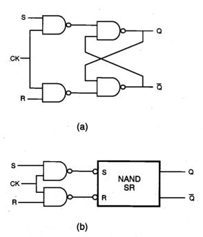
Figure 8.18. (a) Gate-level schematic of the clocked NAND-based SR latch circuit, with active high inputs. (b) Partial block diagram representation of the same circuit.
