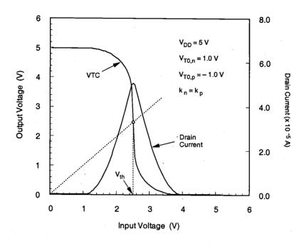
Figure 5.23. Typical VTC and the power supply current of a CMOS inverter circuit.
