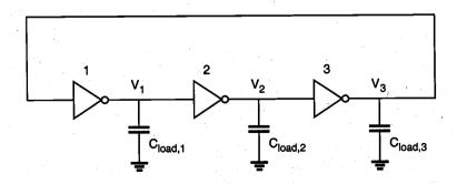
Figure 6.9. Three-stage ring oscillator circuit consisting of identical inverters.
