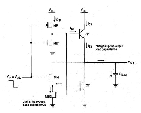
Figure 12.25. BiCMOS inverter during transient output pull-up event. The active devices in the circuit are highlighted (darker).
