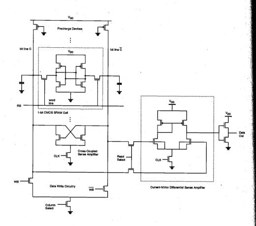
Figure 10.34. Complete circuit diagram of a CMOS static RAM column with data write and data read circuitry.
