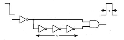
Figure 16.8. A pulse-generation circuit using a delay chain of three inverters.
