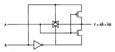
Figure 7.39. Six-transistor CMOS TG implementation of the XOR function.
