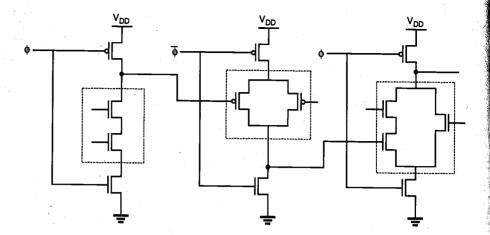
Figure 9.38. NORA CMOS logic circuit example.
