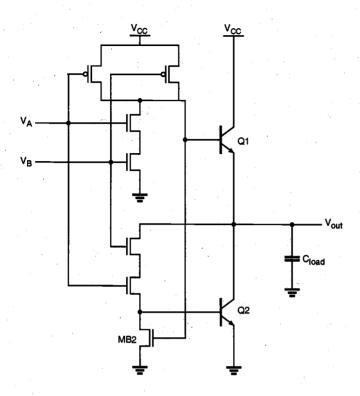
Figure 12.31. Circuit diagram of the BiCMOS NAND2 gate.
