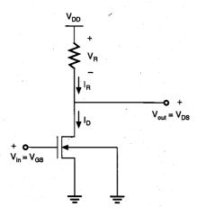
Figure 5.7. Resistive-load inverter circuit.
