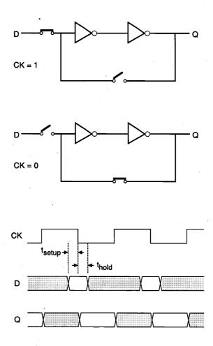
Figure 8.28. Simplified schematic view and the corresponding timing diagram of the CMOS D-latch circuit, showing the setup time and the hold time.
