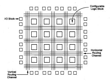
Figure 14.10. General architecture of Xilinx FPGAs.
