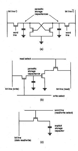
Figure 10.36. Various configurations of the dynamic RAM cell. (a) Four-transistor DRAM cell with two storage nodes. (b) Three-transistor DRAM cell with two bit lines and two word lines. (c) One-transistor DRAM cell with one bit line and one word line.
