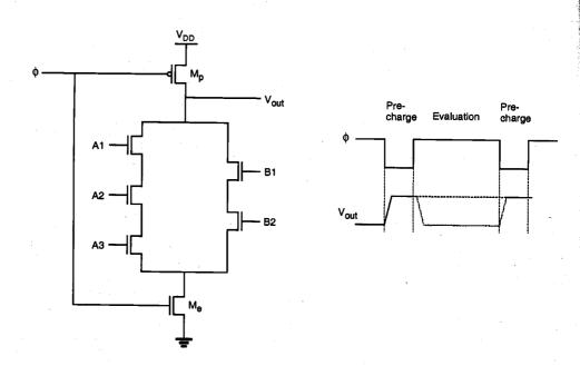
Figure 9.26. Dynamic CMOS logic gate implementing a complex Boolean function.
