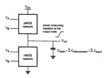
Figure 11.2. Generic representation of a CMOS logic gate for switching power calculation.
