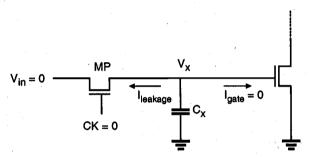
Figure 9.8. Charge leakage from the soft node.
