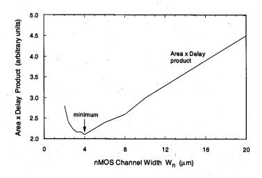
A practical measure used for quantifying design quality is the (Area  $\times$  Delay) product, which takes into account the silicon-area cost of transistor sizing for delay reduction. While the propagation delay asymptotically approaches a limit value for increasing channel widths, the (Area  $\times$  Delay) product exhibits a clear minimum around  $W_n = 4 \, \mu m$ , indicating the optimum choice both in terms of speed and overall silicon area.
