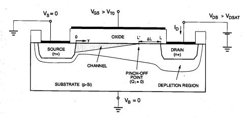
Figure 3.19. Channel length modulation in an n-channel MOSFET operation in saturation mode.
