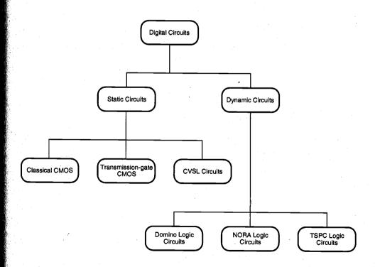
Figure 1.5. Classification of CMOS digital circuit types.
