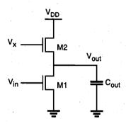
Figure 9.11. Enhancement-type circuit in which the output node is weakly driven.
