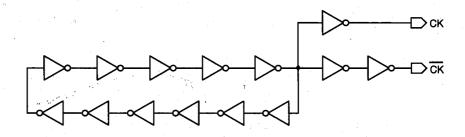
Figure 13.19. Simple on-chip clock generation circuit using a ring oscillator.
