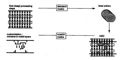
Figure 14.13. Basic processing steps required for gate array implementation.
