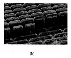
Figure 10.44. (a) Typical one-transistor (1-T) DRAM cell with its access lines. (b) SEM photograph of a stacked-capacitor DRAM cell structure.
