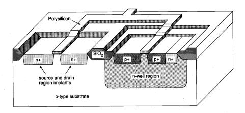
Using a set of two masks, the n+ and p+ regions are implanted into the substrate and Figure 2.8. into the n-well, respectively. Also, the ohmic contacts to the substrate and to the n-well are implanted in this process step. After Atlas of IC Technologies, by W. Maly [1].
