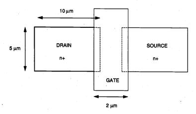
Note that both the source and the drain diffusion regions are surrounded by p<sup>+</sup> channel-stop diffusion. The substrate is biased at 0 V. Assuming that the drain voltage is changing from 0.5 V to 5 V, find the average drain-substrate junction capacitance  $C_{db}$ .
