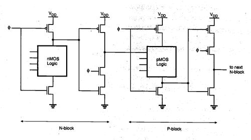
Figure 9.41. A pipelined true single-phase clock CMOS system.
