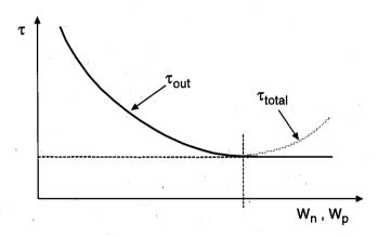
Figure 12.2. Propagation delay of the CMOS buffer vs. transistor size in the output stage.
