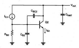
Figure 12.29. Equivalent circuit used for the pull-down delay analysis.
