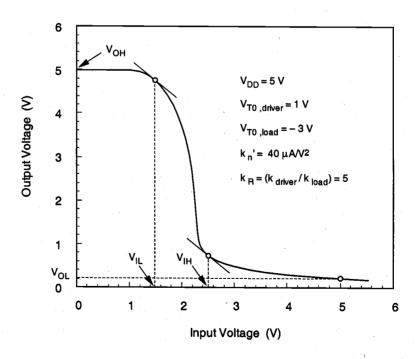
Figure 5.13. Typical VTC of a depletion-load inverter circuit.
