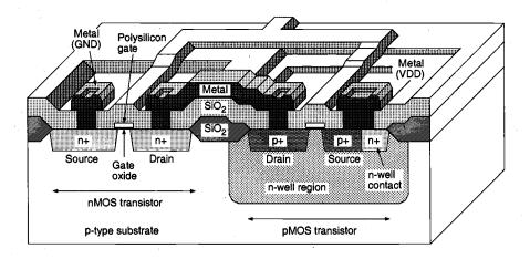
Figure 2.11. The composite layout and the resulting cross-sectional view of the chip, showing one nMOS and one pMOS transistor (in the n-well), and the polysilicon and metal interconnections. The final step is to deposit the passivation layer (for protection) over the chip, except over wire-bonding pad areas. After Atlas of IC Technologies, by W. Maly [1].
