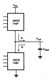
Figure 6.29. Generalized CMOS logic circuit.
