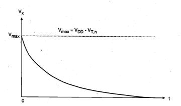
Variation of  $V_r$  as a function of time during logic "0" transfer. Figure 9.7.
