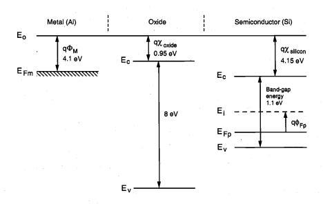
Figure 3.3. Energy band diagrams of the components that make up the MOS system.
