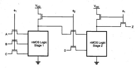
Figure 9.20. General circuit structure of ratioed synchronous dynamic logic.
