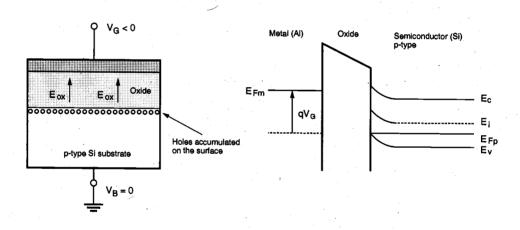
Figure 3.5. The cross-sectional view and the energy band diagram of the MOS structure operating in accumulation region.
