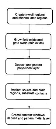
Figure 2.1. Simplified process sequence for the fabrication of the n-well CMOS integrated circuit with a single polysilicon layer, showing only major fabrication steps.
