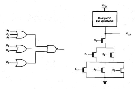
Figure 7.25. An OR-AND-INVERT (OAI) gate, and the corresponding pull-down net.
