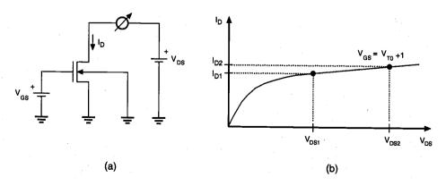
*Figure 3.23.* (a) Test circuit arrangement and (b) measured data for experimental determination of the channel length modulation coefficient  $\lambda$ .
