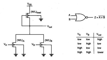
A two-input depletion-load NOR gate, its logic symbol, and the corresponding truth table. Note that the substrates of all transistors are connected to ground.
