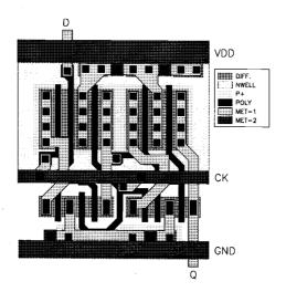
Figure 9.43. Mask layout of the TSPC-based DFF circuit.
