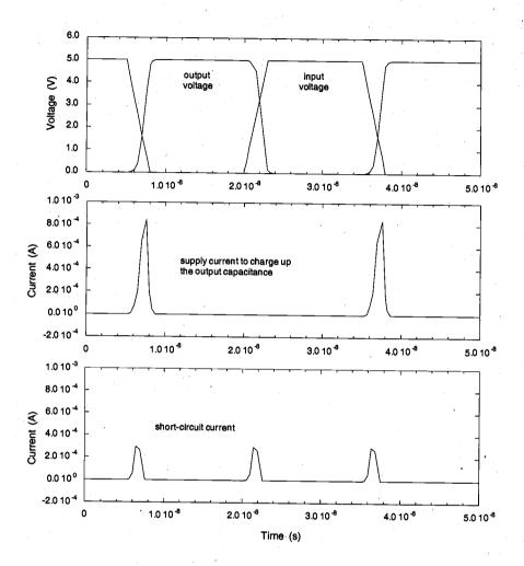
Figure 11.5. Input-output voltage waveforms, the supply current used to charge up the load capacitance and the short-circuit current in a CMOS inverter with small capacitive load. The total current drawn from the power supply is the sum of both current components.
