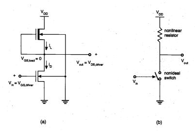
Figure 5.12. (a) Inverter circuit with depletion-type nMOS load. (b) Simplified equivalent circuit consisting of a nonlinear load resistor and a nonideal switch controlled by the input.
