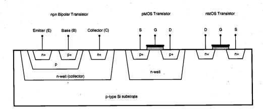
Figure 12.4. Simplified cross-section showing an npn bipolar transistor, an n-channel MOS transistor, and a p-channel MOS transistor fabricated on the same p-type silicon substrate. Notice that many standard CMOS process steps can be used to create bipolar and MOS transistors side-by-side on the chip.
