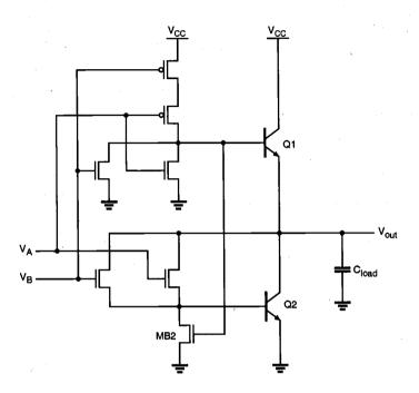
Figure 12.30. Circuit diagram of the BiCMOS NOR2 gate.
