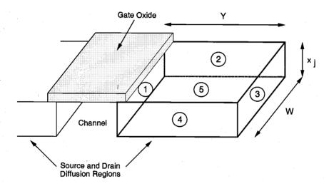
Figure 3.33. Three-dimensional view of the n<sup>+</sup> diffusion region within the p-type substrate.
