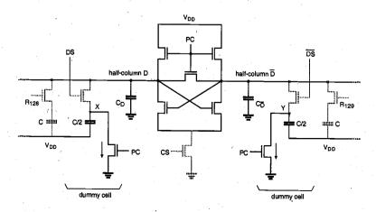
Figure 10.46. The half-columns are being charged-up during the precharge phase.
