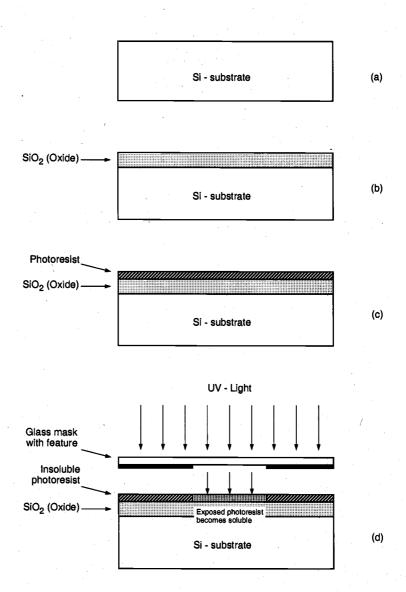
Figure 2.2. Process steps required for patterning of silicon dioxide.
