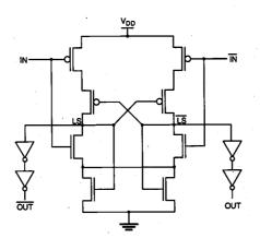
Figure 13.16. Receiver circuit designed to sense, latch, and level-shift differential data.
