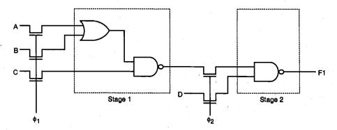
Figure 9.17. A two-stage synchronous complex logic circuit example.
