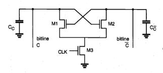
Figure 10.33. Cross-coupled nMOS sense amplifier circuit.
