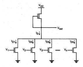
Figure 7.3. Generalized n-input NOR gate.
