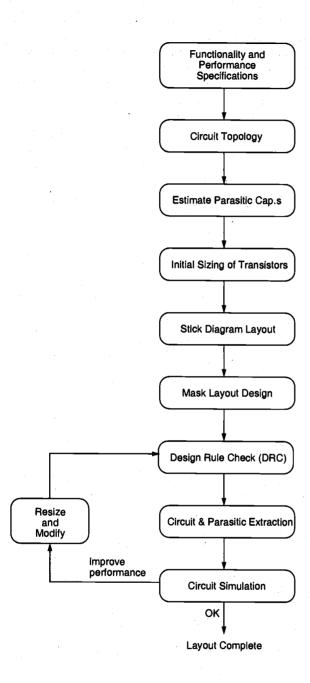
Figure 2.13. Typical design flow for the production of a mask layout.
