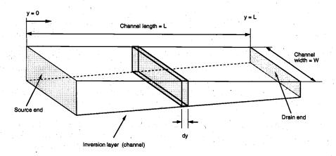
Figure 3.16. Simplified geometry of the surface inversion layer (channel region).
