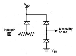
Figure 13.3. ESD protection network example.
