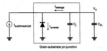
Figure 9.10. Equivalent circuit used for analyzing the charge leakage process.
