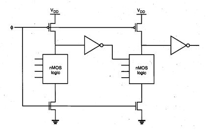
Figure 9.29. Cascaded domino CMOS logic gates.
