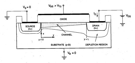
Figure 3.15. Cross-sectional view of an n-channel transistor, operating in linear region.
