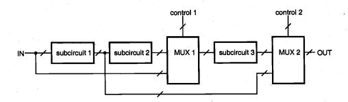
Figure 16.5. Partition-and-mux method for large circuits.
