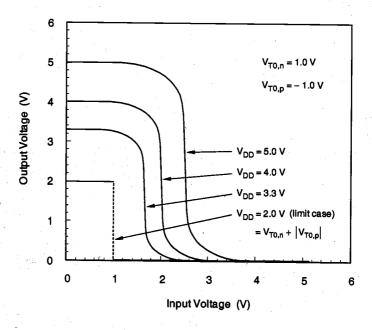
Figure 5.25. Voltage transfer characteristics of a CMOS inverter, obtained with different power supply voltage levels.
