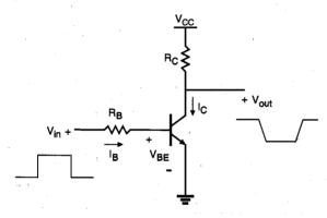
Figure 12.17. BJT inverter with ideal pulse voltage waveform applied to the input.
