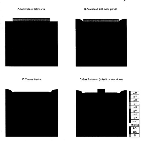
**PLATE 1:** Fabrication steps for an nMOS transistor on p-type silicon substrate.
