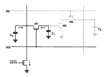
**Figure 10.42.** Both  $C_1$  and  $C_2$  are discharged via M1 and the data write transistor during the write "0" sequence.
