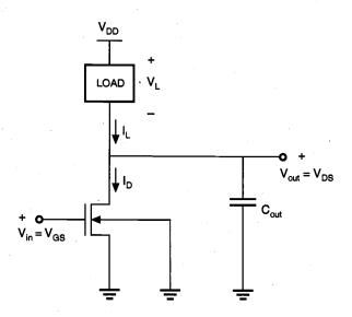
Figure 5.3. General circuit structure of an nMOS inverter.
