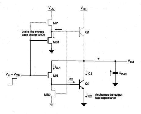
Figure 12.28. BiCMOS inverter during a transient output pull-down event. The active devices in the circuit are highlighted (darker).
