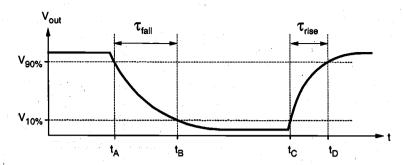
Figure 6.4. Output voltage rise and fall times.
