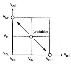
Figure 8.5. Phase-plane representation of the bistable circuit behavior.
