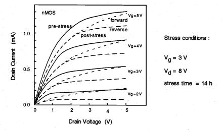
Figure 3.28. Typical drain current vs. drain voltage characteristics of an n-channel MOS transistor before and after hot-carrier induced oxide damage.
