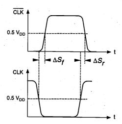
Figure 15.20. Definition of rising and falling clock skews.
