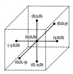
Figure 15.10. Central composite design for n = 3.
