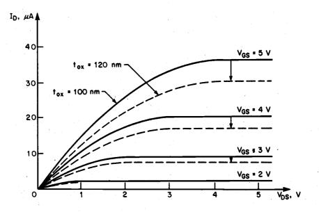
Figure 4.4. Variation of the drain current with model parameter TOX, for the LEVEL1 model (Copyright © 1988 by McGraw-Hill, Inc.).
