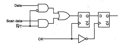
Figure 16.10. Scan-based design of an edge-triggered D flip-flop.
