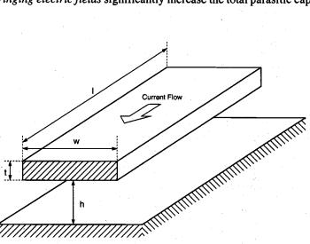
Figure 6.16. Interconnect segment running parallel to the surface, which is used for parasitic resistance and capacitance estimations.
