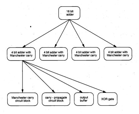
Figure 14.8. Structural hierarchy of the 16-bit adder circuit.
