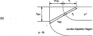
Figure 3.25. (a) Simplified geometry of the MOSFET channel region, with gate-induced bulk depletion region and the pn-junction depletion regions. (b) Close-up view of the drain diffusion edge.
