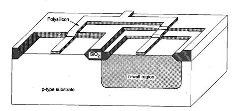
Figure 2.7. The polysilicon layer is deposited using chemical vapor deposition (CVD) and patterned by dry (plasma) etching. The created polysilicon lines will function as the gate electrodes of the nMOS and the pMOS transistors and their interconnects. Also, the polysilicon gates act as self-aligned masks for the source and drain implantations that follow this step. After Atlas of IC Technologies, by W. Maly [1].
