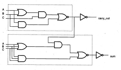
Figure 1.7. Gate-level schematic of the one-bit full-adder circuit.
