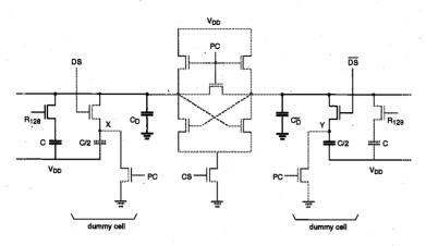
Figure 10.47. Two complementary column voltages are determined through charge sharing, on the one side between the selected storage cell and the half-column capacitance, on the other side between the dummy cell and the other half-column capacitance.
