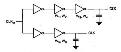
Figure 15.19. Clock distribution circuit.
