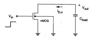
Figure 6.5. Equivalent circuit of the CMOS inverter during high-to-low output transition.
