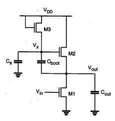
Figure 9.12. Dynamic bootstrapping arrangement to boost  $V_x$  during switching.
