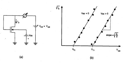
**Figure 3.22.** (a) Test circuit arrangement and (b) measured data for experimental determination of the parameters  $k_n$ ,  $V_{T0}$ , and  $\gamma$ .
