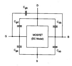
Figure 3.30. Lumped representation of the parasitic MOSFET capacitances.
