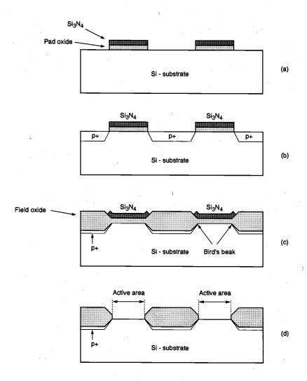
Figure 2.5. Basic steps of the LOCOS process to create oxide isolation around active areas.
