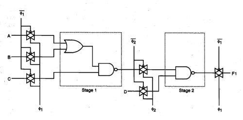
Figure 9.23. Typical example of dynamic CMOS transmission gate logic.
