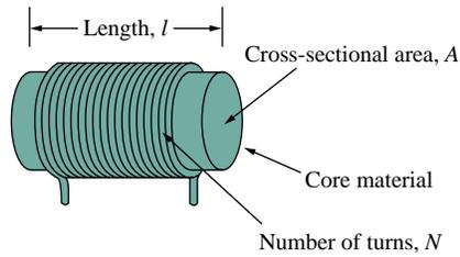
Figure 6.21 Typical form of an inductor.
