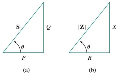
Figure 11.21 (a) Power triangle, (b) impedance triangle.
