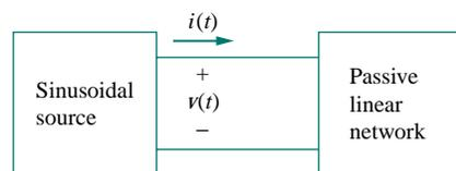
Figure 11.1 Sinusoidal source and passive linear circuit.
