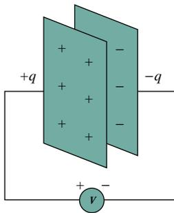
Figure 6.2 A capacitor with applied voltage  $v$ .
