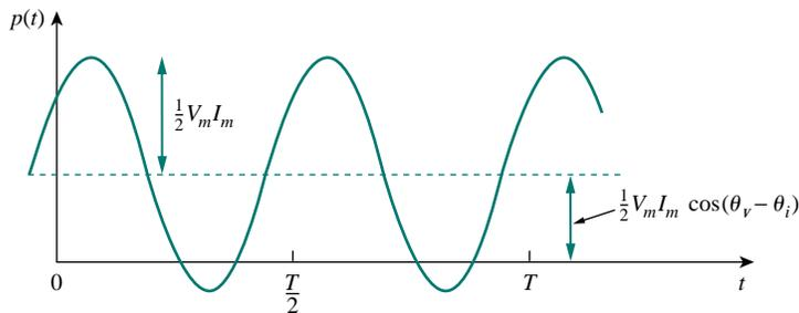
Figure 11.2 The instantaneous power  $p(t)$  entering a circuit.
