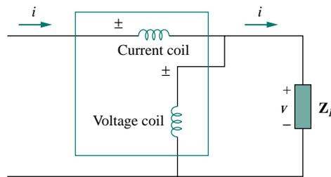
Figure 11.31 The wattmeter connected to the load.
