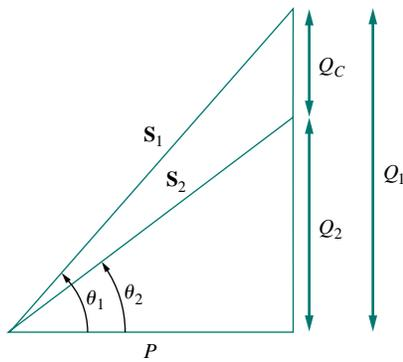
Figure 11.29 Power triangle illustrating power factor correction.
