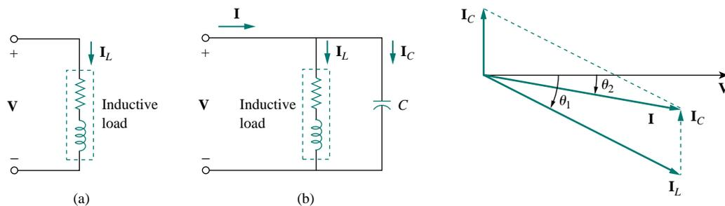
**Figure 11.27** Power factor correction: (a) original inductive load, (b) inductive load with improved power factor.
