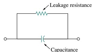
**Figure 6.8** Circuit model of a nonideal capacitor.
