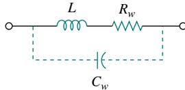
Figure 6.26 Circuit model for a practical inductor.
