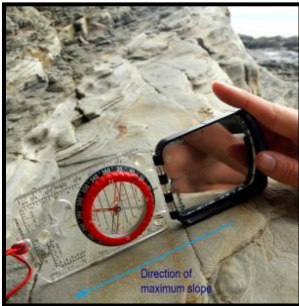
Figure 2 Measurement of strike (left) and dip (right) using a geological compass with a clinometer. [SE]
