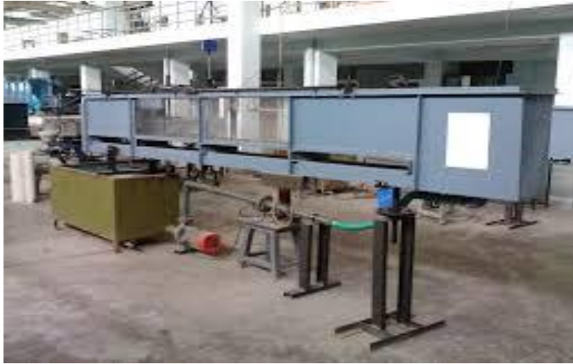
Experimental setup of a rectangular channel for hydraulic jump formation
