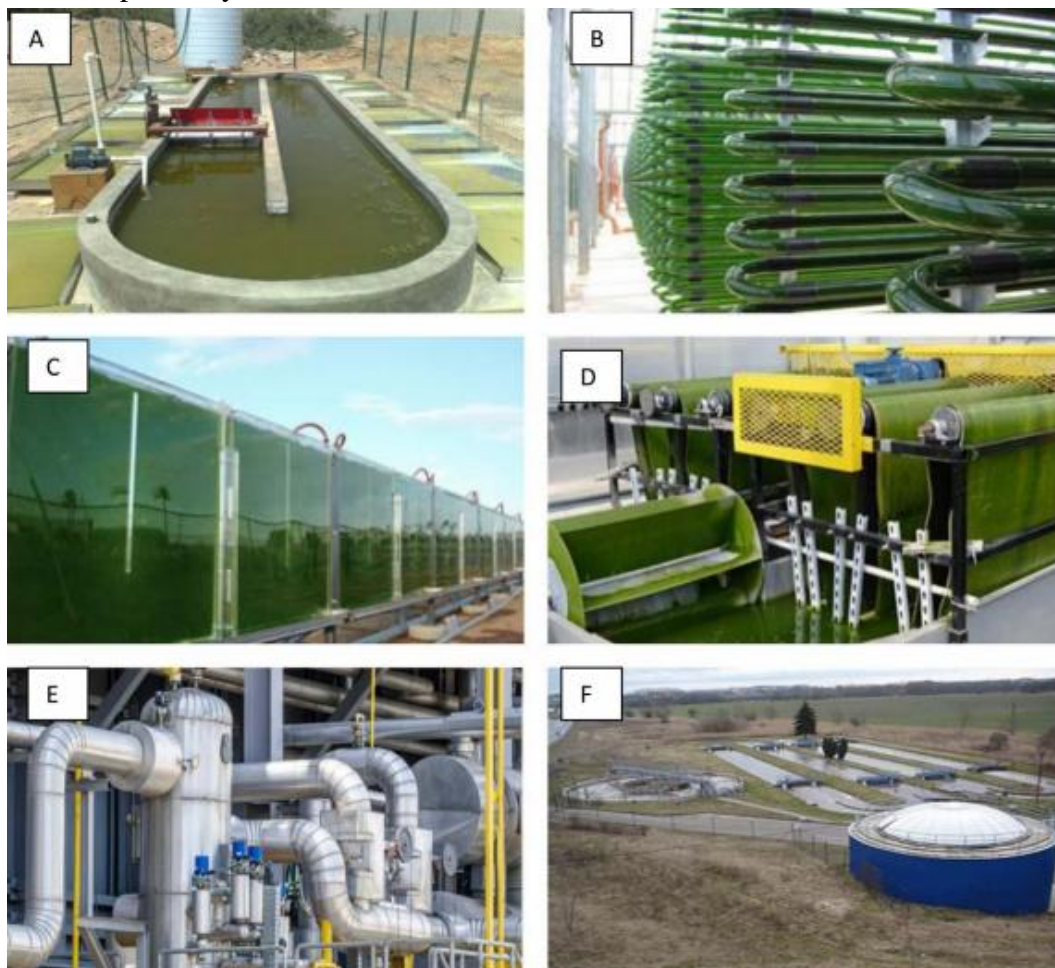
Figure-9: Different systems for algal cultivation A) Open ponds B) Tubular PBRs C) Flat PBRs D) Biofilm based PBRs E) Fermentor cultivation F) algal biomass cultivation using waste water. (PBRs: Photo Bioreactor Systems)
