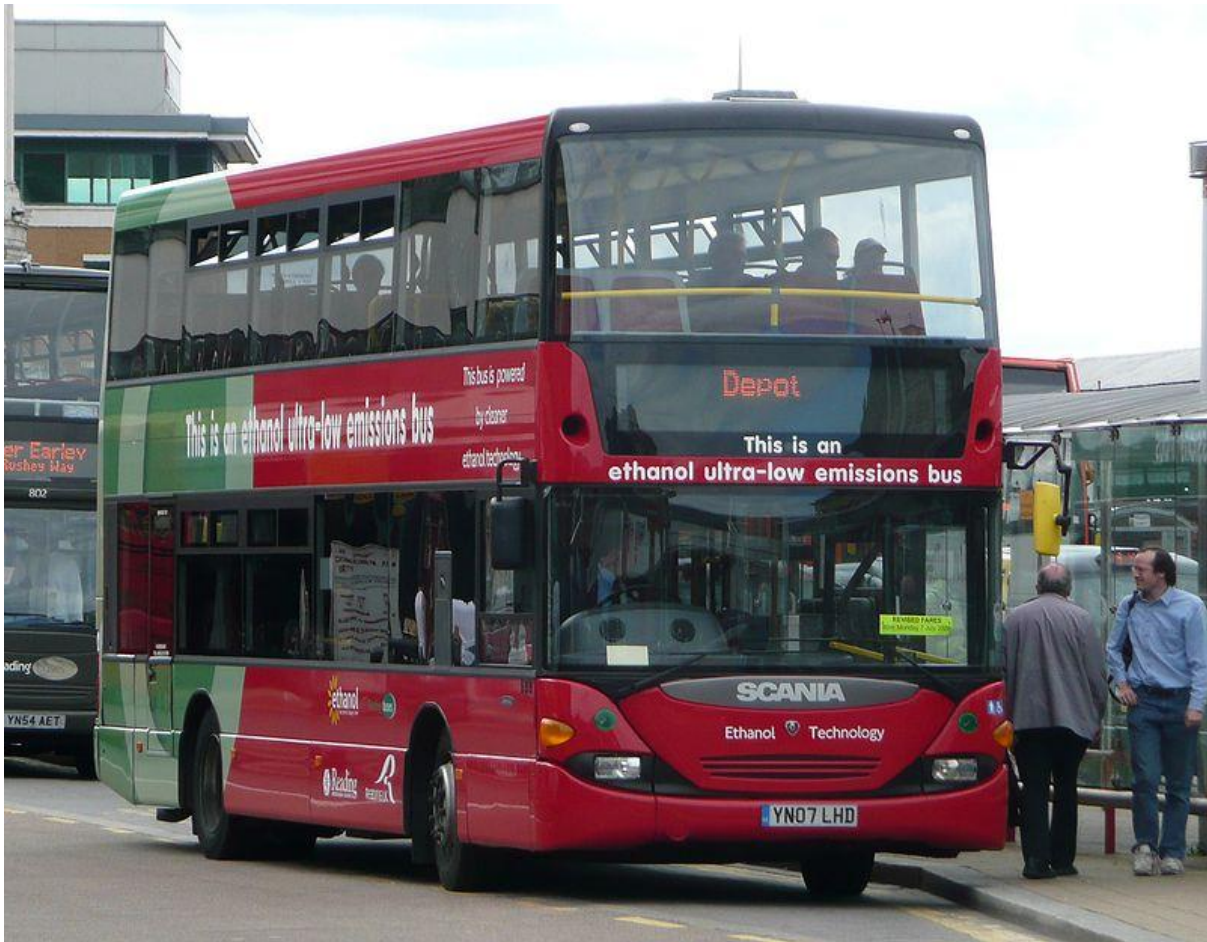
An example of an ethanol powered bus. This is a Scania OmniCity which has been touring the United Kingdom, which does not use the fuel widely. A larger fleet of similar buses entered service in Stockholm in 2008.
